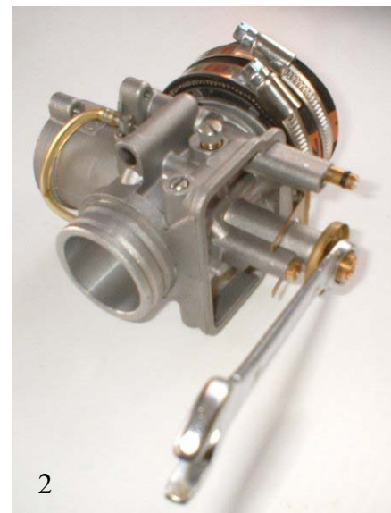
Best method of removal of brass nut is to place one hand on carb body and push down on spanner
